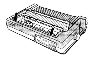
4. Secure the case with **the** three screws.
